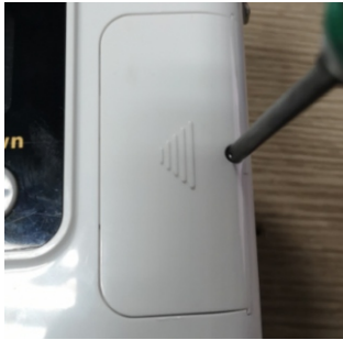
Step 1: Screw out the screws on the battery house cover with a cross screwdriver.
