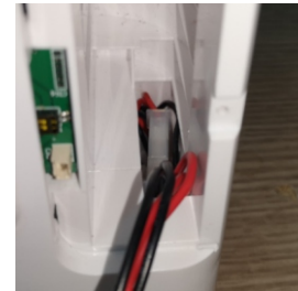
Step 7: The connector is first put into the groove at the bottom of the battery house.
